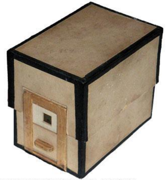
mat board pinhole camera, circa 1972
